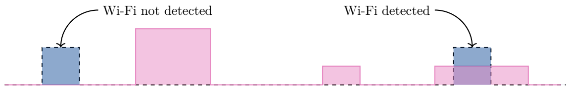
FIGURE 3.12: RSSI scanning in blue tries to detect Wi-Fi signal in rose.
