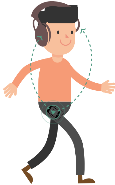
FIGURE 2.4: Illustration of the wireless propagation through human body problem: here, in the worst-case scenario, the smartphone located in the right pocket must communicate with the left earbud, meaning that the signal has to get through about 70 cm of the human body for a typical 1.8 m tall person. This image is an adapted version of the Man Walking Cartoon Vector provided by VideoPlasty under CC BY-SA 4.0 license.
